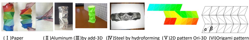
Fig.2 2 types of 2D pattern for RSC, 3D RSC by Ori3D & Add-3D and by hydroforming
